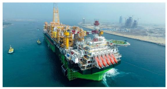
The massive (330mx 61mx 33.5m) Egina Floating Production Storage and Offloading (FPSO) vessel is a spread moored FPSO connected through a subsea production system to 44 wells (21 oil producers and 23 water injectors) via umbilicals, flow lines and risers. Source:
